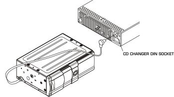
When you want to play the CD changer, plug the CD changer DIN into the socket of the back of the car audio unit.
